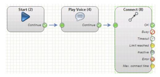
If a required parameter is not provided, the object turns red and an error symbol is shown. Yellow signifies objects where a recommended setting is missing, a yellow warning symbol is shown. Information on the error or recommended parameter settings is shown when you move the mouse cursor over the error or warning symbol.
